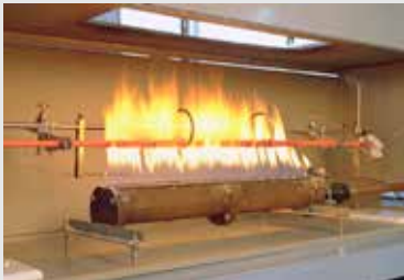
Fire Resistant Test with Fire Alone
